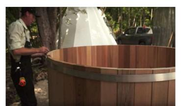
Slip the assembled band over the tub.
