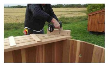
To assemble benches, rest the benches on top of the tub to attach the bench-end supports.
