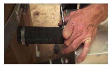
Slide the heater into place and hook up the back of the heater to the heater hoses.
