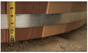
Slide band to the bottom of the tub.
