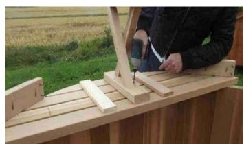
Secure the centre support to the bottom of the bench using the provided 2" screws .
